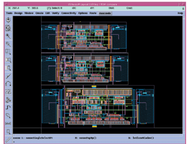
Figure 4 – Three Derivatives from One Layout Topology (Template)
